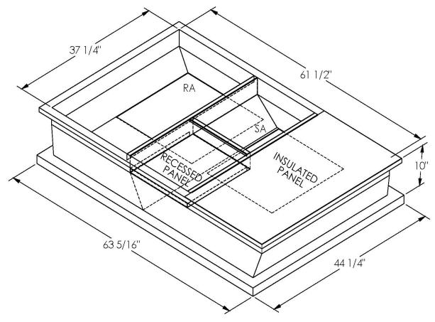
ONE PIECE WELDED CONSTRUCTION
