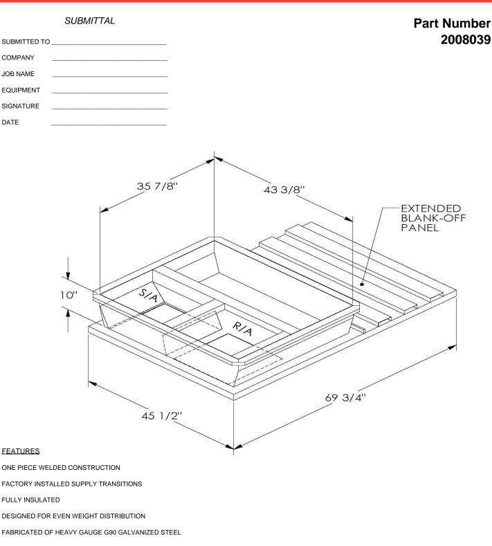
ALL WELDS SPRAYED WITH GALVANIZING COMPOUND
