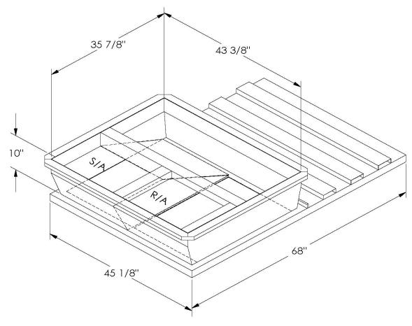
ONE PIECE WELDED CONSTRUCTION
