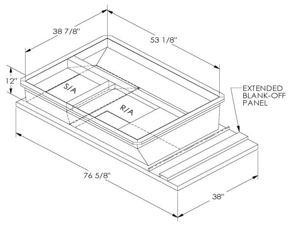
ONE PIECE WELDED CONSTRUCTION
