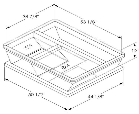
ONE PIECE WELDED CONSTRUCTION
