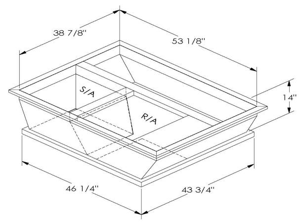
ONE PIECE WELDED CONSTRUCTION
