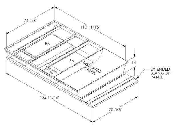
ONE PIECE WELDED CONSTRUCTION
