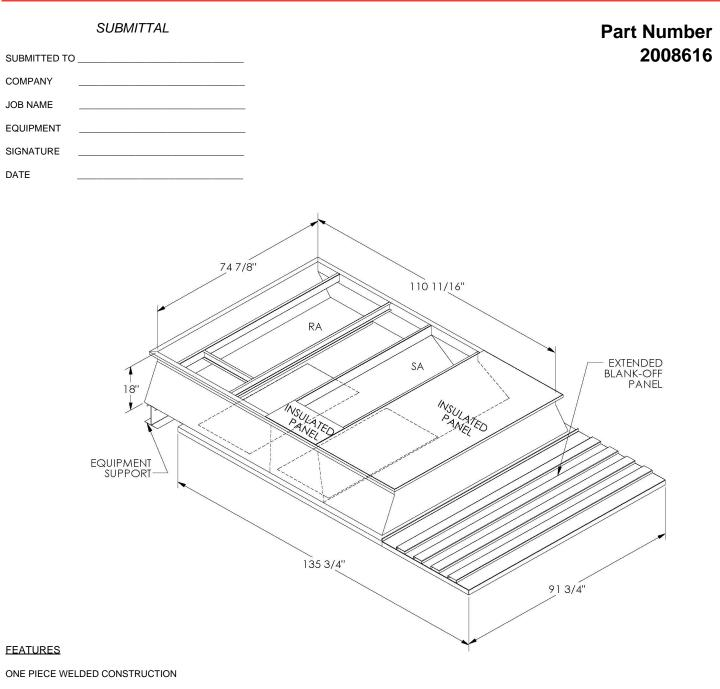
FACTORY INSTALLED SUPPLY TRANSITIONS
