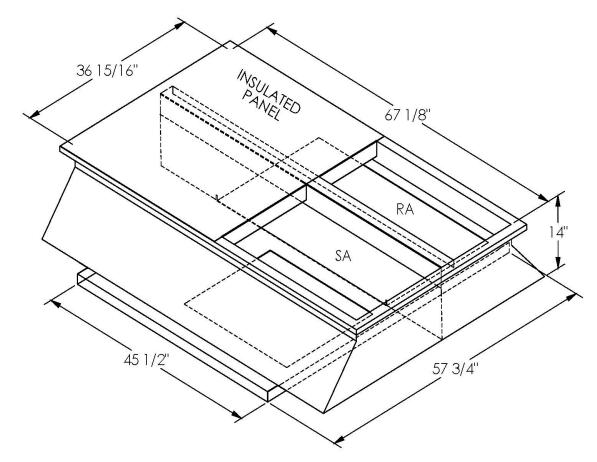
ONE PIECE WELDED CONSTRUCTION
