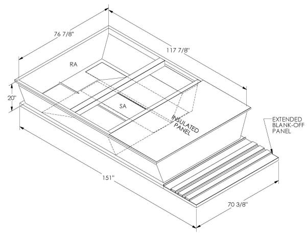
ONE PIECE WELDED CONSTRUCTION
