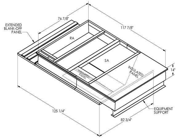
ONE PIECE WELDED CONSTRUCTION
