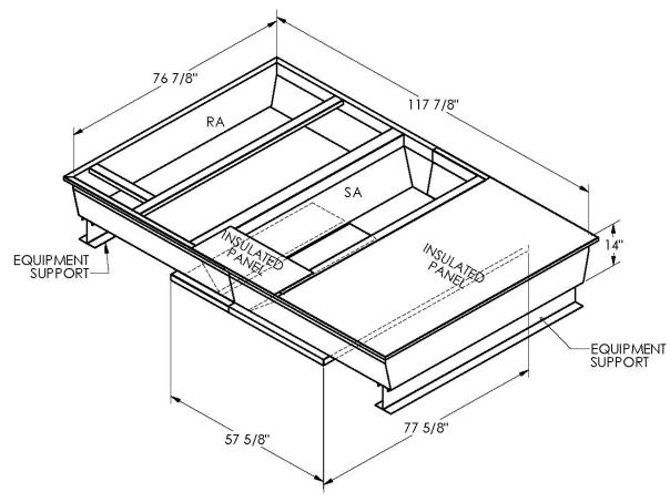
ONE PIECE WELDED CONSTRUCTION
