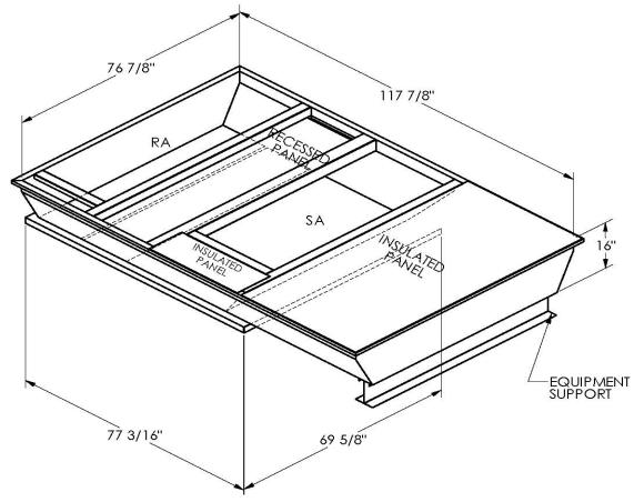
ONE PIECE WELDED CONSTRUCTION
