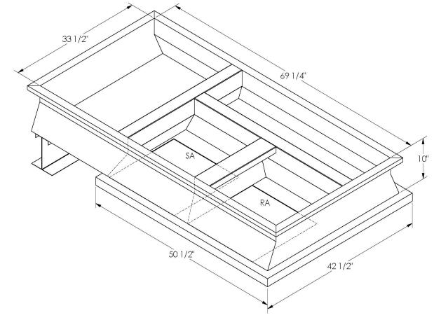
ONE PIECE WELDED CONSTRUCTION
