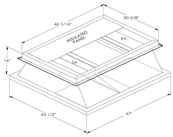
ONE PIECE WELDED CONSTRUCTION
