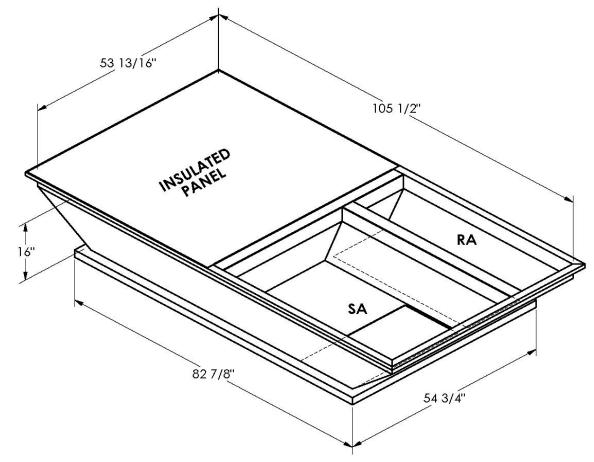
ONE PIECE WELDED CONSTRUCTION
