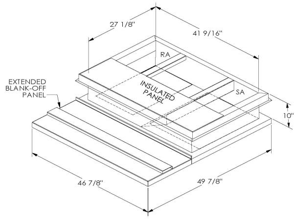
ONE PIECE WELDED CONSTRUCTION
