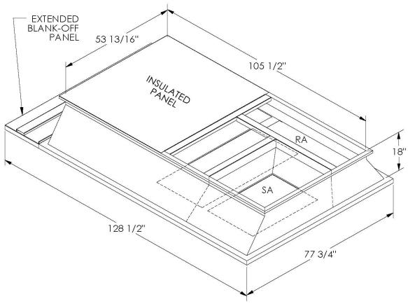
ONE PIECE WELDED CONSTRUCTION
