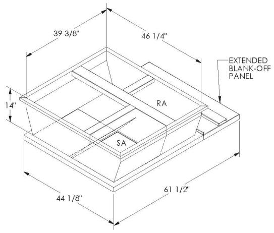
ONE PIECE WELDED CONSTRUCTION
