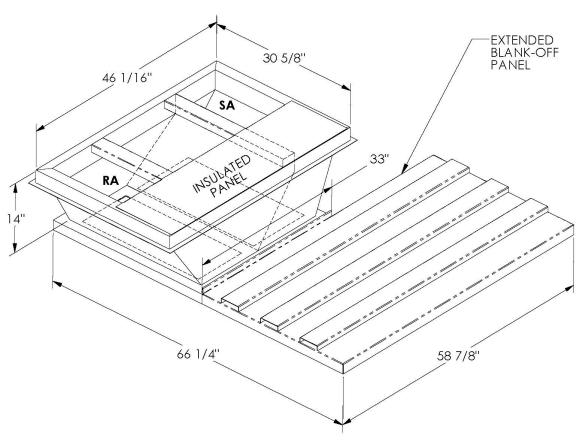
ONE PIECE WELDED CONSTRUCTION
