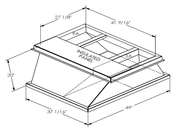
ONE PIECE WELDED CONSTRUCTION
