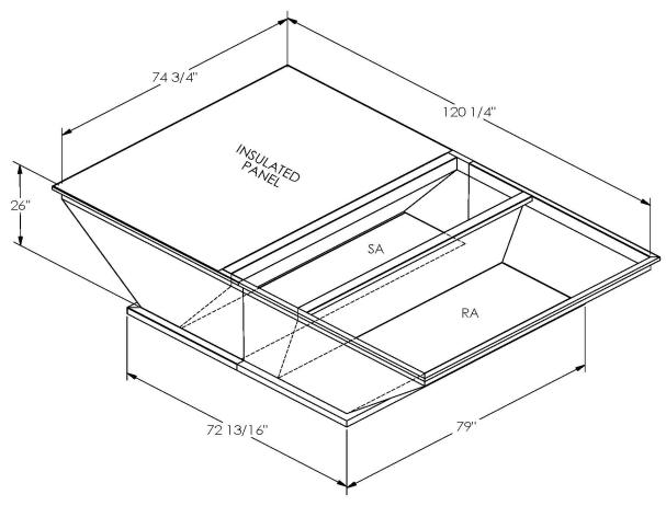
ONE PIECE WELDED CONSTRUCTION
