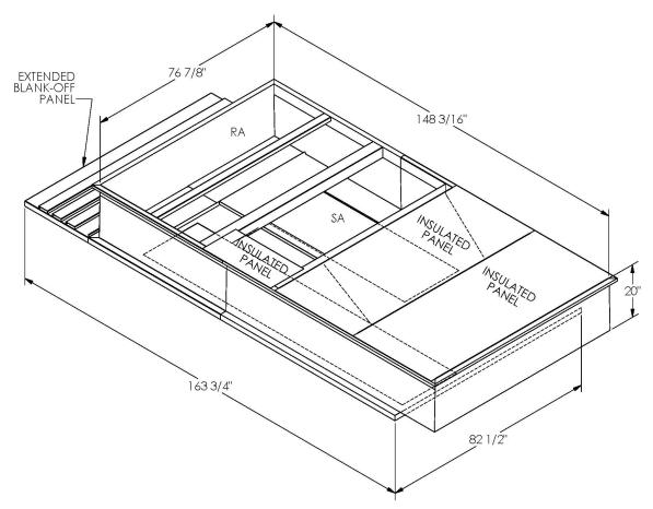
ONE PIECE WELDED CONSTRUCTION
