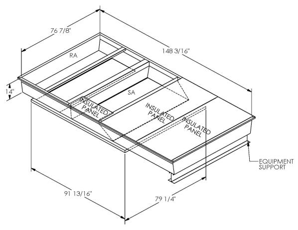
ONE PIECE WELDED CONSTRUCTION
