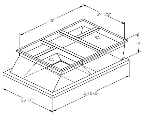
ONE PIECE WELDED CONSTRUCTION
